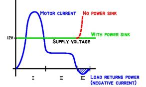
Fig. 1 Typical load current PWM - controlled DC motor
