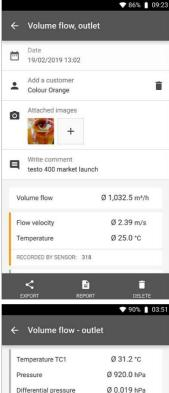
The calculated result of the measurement is displayed under the Customer data, Images and Comments.
