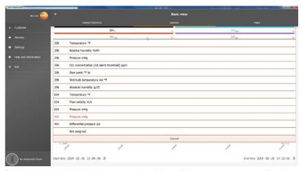
Below the graphic, both the start and end time of the measurement are listed. The information can be changed by clicking on the individual fields with the mouse. The trend graph immediately adapts to the new time selection.
