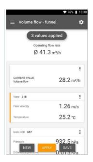
6 Apply: the current reading is applied.
