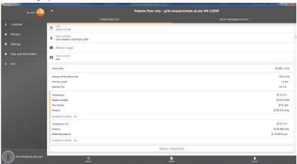
Via the three icons in the footer, the measurement results can be saved as a .csv /.json file or as a PDF report on the computer or permanently deleted
