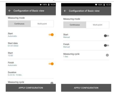
Click on Apply Configuration to start the measurement (with a scheduled start time).
