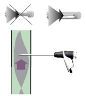
The thermocouple of the flue gas probe must not lie against the probe cage.
