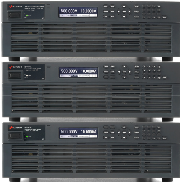
Figure 5. Parallel operation for more power
