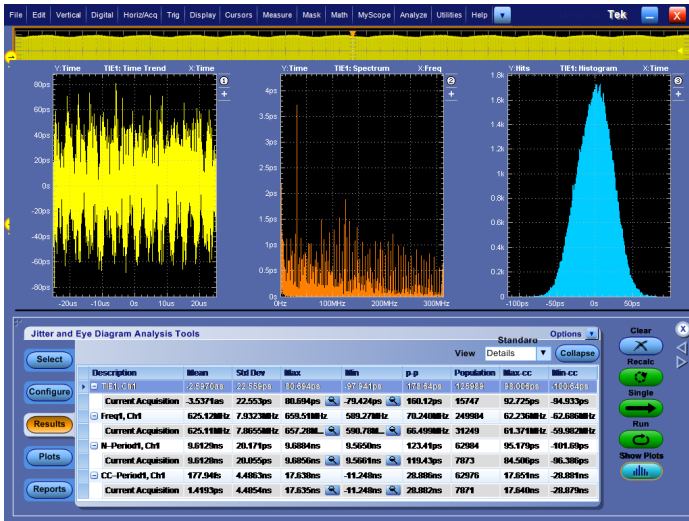
Jitter analysis - TIE jitter/timing analysis of 622 Mb/s signal
