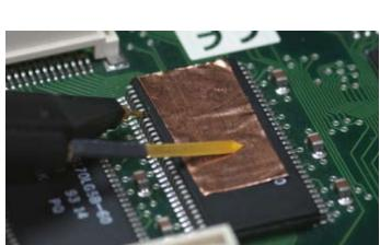
Very short ground connections can be established with the ground blade and the copper pads – for signal true measurements on ICs.
